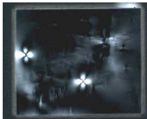
Figure 1. Birefringence seen in crossed-polarizers of two four-petalled defects in CVD diamond. The plane of view is (001). The horizontal and vertical axes lie along \langle 100 \rangle and the polarizers lie along \langle 110 \rangle . Figure provided by Martineau.
